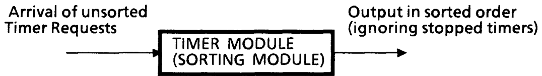
FIGURE 5 - ANALOGY BETWEEN A TIMER AND A SORTING MODULE
