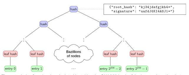
The entry index for a key is calculated by taking the SHA256 hash of the key, and treating that as a 256-bit big endian integer. The value for that key is stored in the leaf node indexed by this number. The tree size is therefore always  $2^{256}$ .
